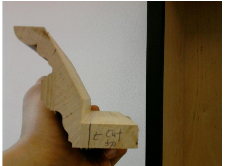
(Cut the back end piece, Leave 1/4-1/2")
