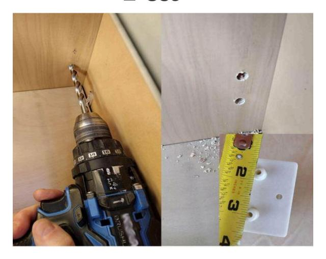
**Step 4:** Pull the rear mounting brackets apart (use some force). Use two ½" screws to secure the bracket rear plates to the height where the roll out tray is desired. Slide the extended part of the bracket back into the rear plate.
